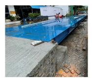
A low profile weighbridge that is versatile and easy to install, the structure is almost identical as the former. But because it is elevated and installed on the ground level, maintenance works are far easier. It also requires minimal and simple civil works.
